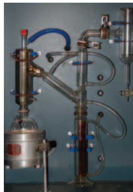
Vacuum Distillation apparatus for Testing Biodiesels Standards
